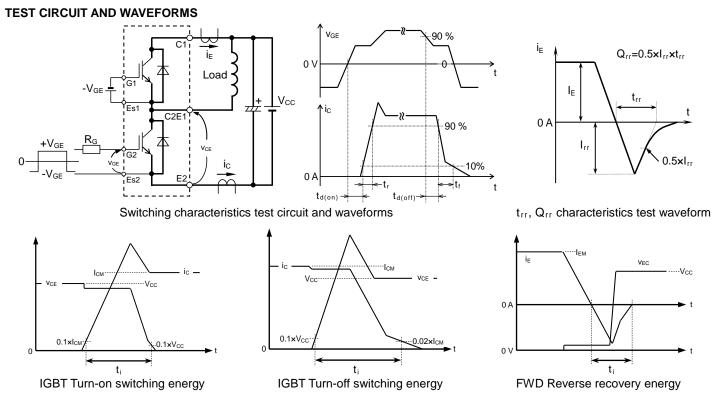
Turn-on / Turn-off switching energy and Reverse recovery energy test waveforms (Integral time instruction drawing)
